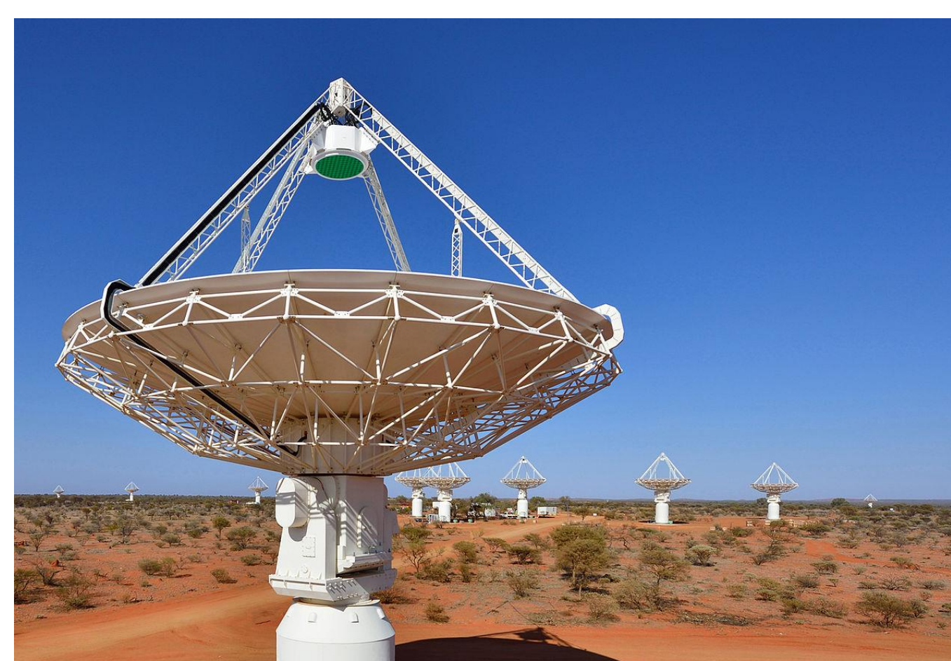
Figure 5: The Rapid ASKAP Continuum Survey (RACS) is the first large-area survey performed with the Australian Square Kilometre Array Pathfinder (ASKAP) telescope. It covers over 34000 sq deg of the sky at \sim 888 \text{MHz} , down to a sensitivity level of \sim 300 \mu\text{Jy} .
